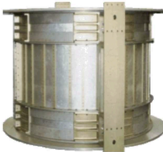
Figure 2.2: The AMS-02 magnet field orientation [6]. The varying direction of the magnetic field in the material allowed the flux to be returned primarily within the material allowing for a negligible external field. A quite uniform field is generated in the inner part of the volume. The magnet blocks and the coordinate system are shown in the left picture. The arrows in the right exhibit the magnetization direction \alpha .
