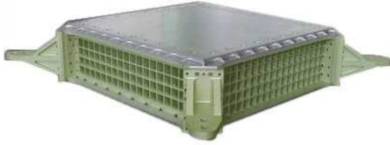
Figure 2.16: The ECAL before the PMTs installation on the lateral slots (visible on the detector sides).
