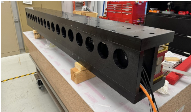
Figure 1: An APS 2.4-meter-long FNAPU with a 27-mm period length.
