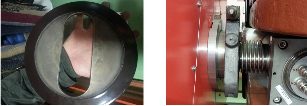
FIGURE 2.15: Flange disk with ceramic layer (left); one of the isolated PS flange provided by RF bypass installed in the ring (right).
