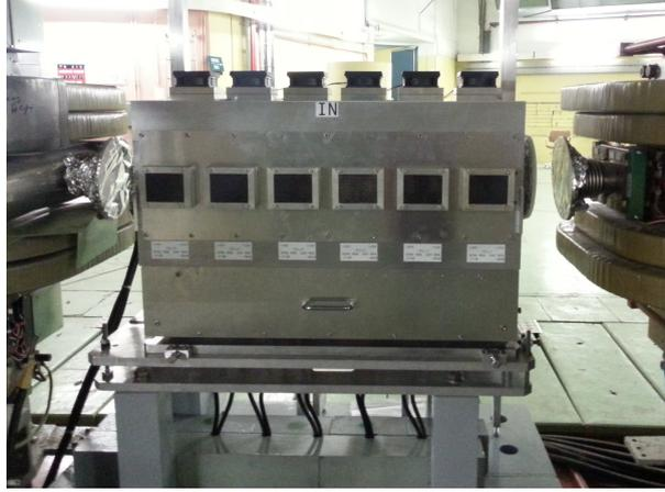
FIGURE 5.20: Longitudinal damper after installation in SS01 of the PS ring.
