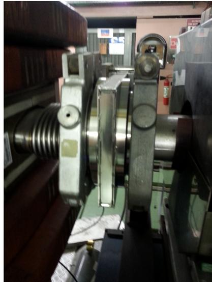
FIGURE 2.13: Picture of a PS sector valve.
