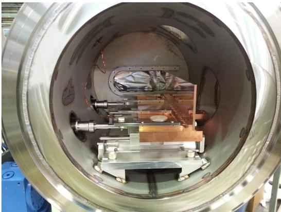
FIGURE 5.4: Inside view with blade and support table installed.
