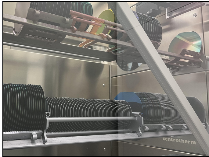
Figure 4.1.: Photo of the horizontal cluster system (Centrotherm 2000) that deposits poly-Si layers on wafers using the LPCVD technique.
