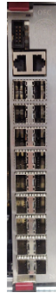
Figure 4. OFC-1 consists of an Arria 5 FPGA, and 18 SFP I/O (4Gbps). Most are used for the 16 ADC module output per crate, and only two are available for output.
