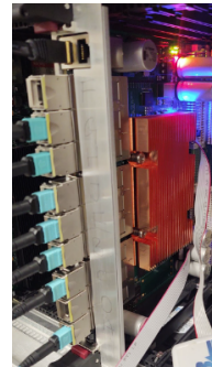
Figure 5. OFC-2 is a major upgrade from the OFC-1. The FPGA is a Stratix X with 8GB of high bandwidth on chip memory. There are 9 QSFP I/O which can send and receive data at 40Gbps.
