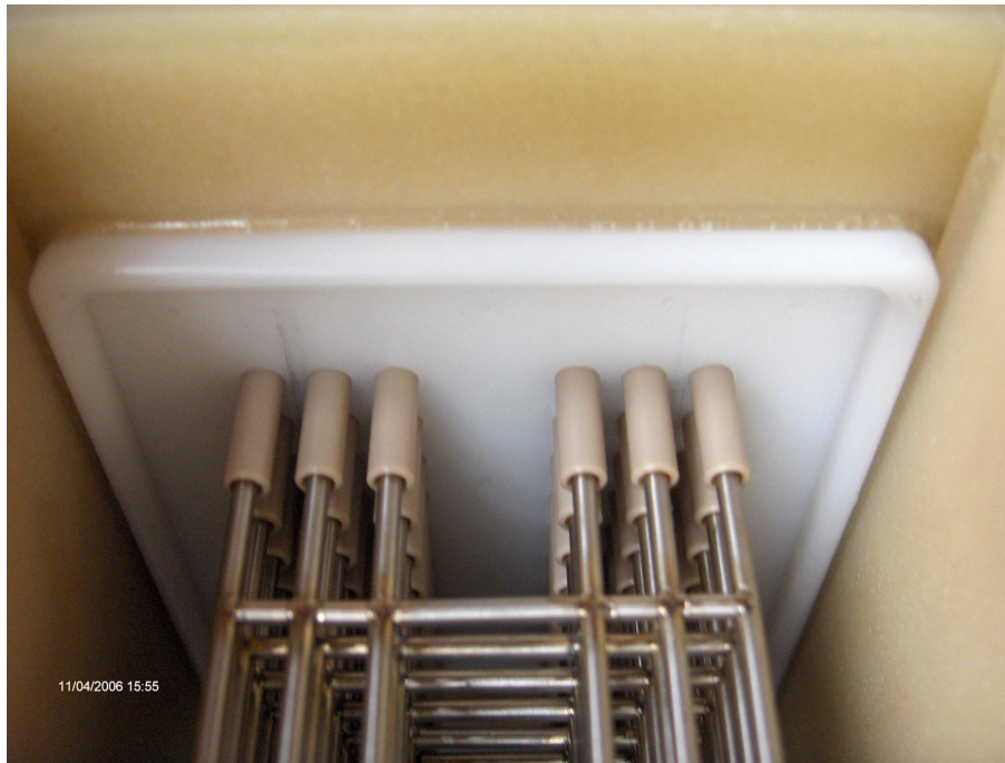
Figure 7.4: The field shaping electrodes fixated in a Polyamid-plate that is inserted in the chamber walls. The electrodes are additionally protected by small insulators made of PEEK.
