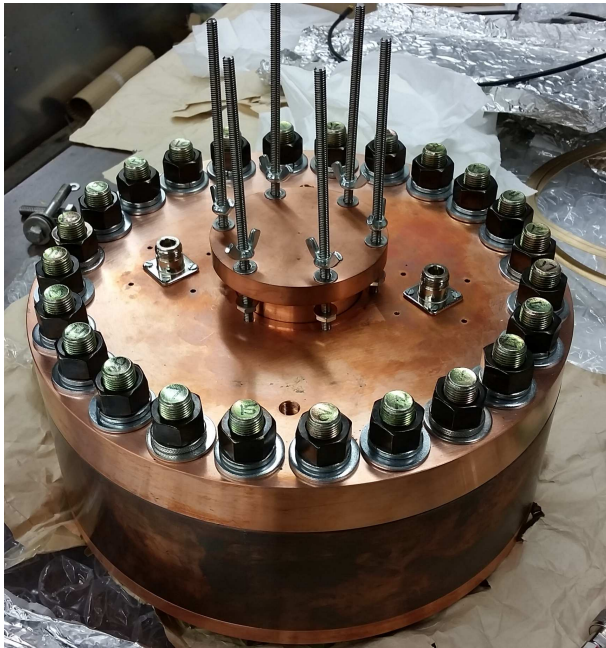
Figure 1: Dielectric sample test cavity fully assembled. Two copper endplates are held to a cylindrical body with 24 bolts. The samples are placed on a cylindrical copper electrode attached to the bottom endplate (not shown). A copper plunger (shown) is fastened in place to make contact with the sample and top endplate. Pickup probe ports are also shown.
