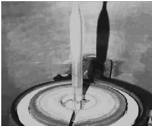
Fig. 6.6. A crystallization chamber with pulled (\text{Lu}_{0.7}\text{-Y}_{0.3})\text{AlO}_3\text{:Ce} crystal
