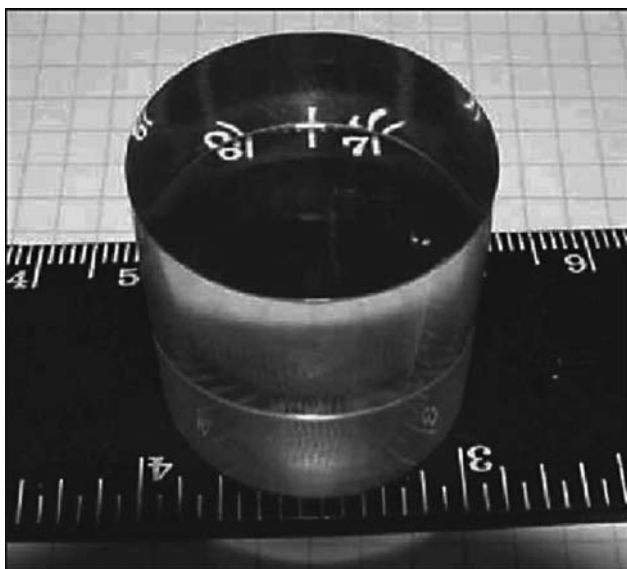
Fig. 6.7. A 1 in (\text{Lu}_{0.7}\text{-Y}_{0.3})\text{AlO}_3\text{:Ce} scintillation crystal for spectrometry applications
