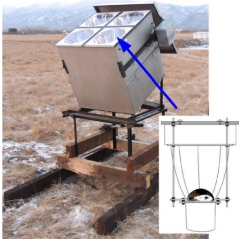
Figure 1. The Tunka-HiSCORE optical station. Additional window: the layout of one PMT segment.
