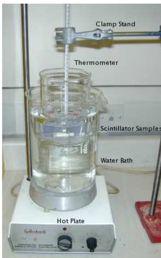
Figure 5.1: Photograph of the apparatus used to measure scintillator solution cloud points.
