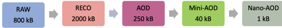
Figure 3.12: Diagram above shows the different types of Data formats utilized by CMS and their estimated sizes for each occurrence. The formats follow a consistent sequence, where, for instance, NanoAOD derives from MiniAOD.
