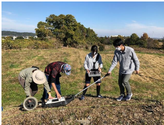
Figure 4: GPR survey on the top of Akiyama Koshinzuka Kofun by high school students and graduated students of archaeology course(left). Dependence of radar reflection intensity on distance from the ground surface z (right). z = 0.6 - 0.7 m (top), z = 1.4 - 1.5 m (middle), z = 2.2 - 2.4 m (bottom).
