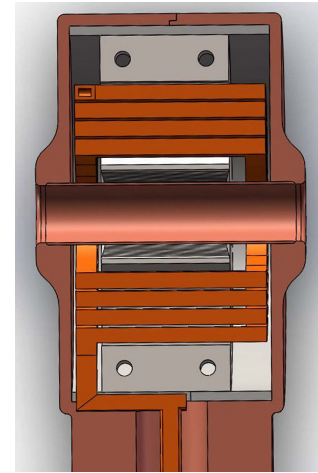
Figure 7: Diagram of the assembly of the quadrupole inside the first DTQ.
