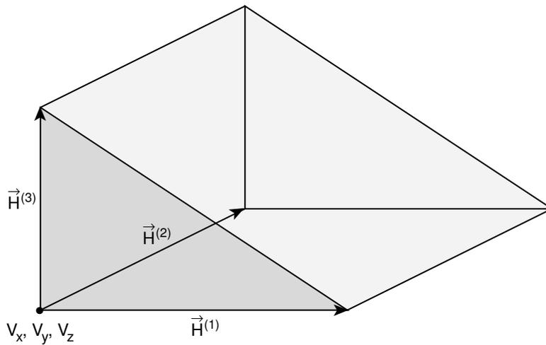
**Fig. 8.8:** Right Angle Wedge (WED or RAW)
