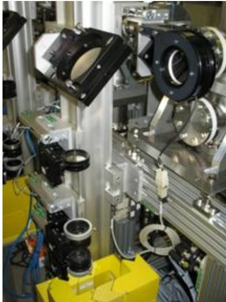
Figure 8.1: In the tomography section of the PITZ beam-line, advanced CCD cameras, well shielded from stray radiation, are used with high-quality remotely-adjustable optics to provide optimum screen images.
