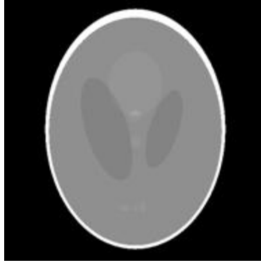
Figure 1.15: The Shepp-Logan phantom [29] is entirely composed of a superposition of simple uniform ellipses, which are specified by their centre coordinates, principal axis lengths, rotation angles and densities.
