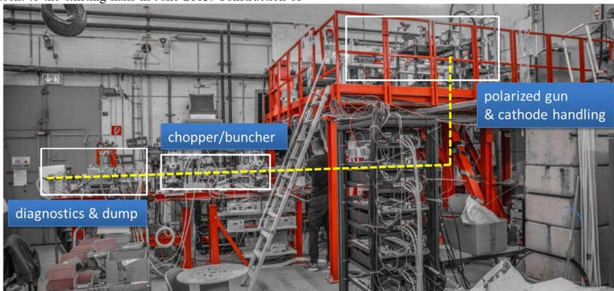
Figure 2: Injector test setup as run until July 2019. The test beamline consisted of the polarized inverted dc gun STEAM and parts of the MELBA LEBT system (chopper, buncher and beam transport). Extensive longitudinal and transverse diagnostics have been set up and used for beam characterization. The way of the electron beam along the beamline is illustrated by the yellow dashed line (photography: MELBA group).
