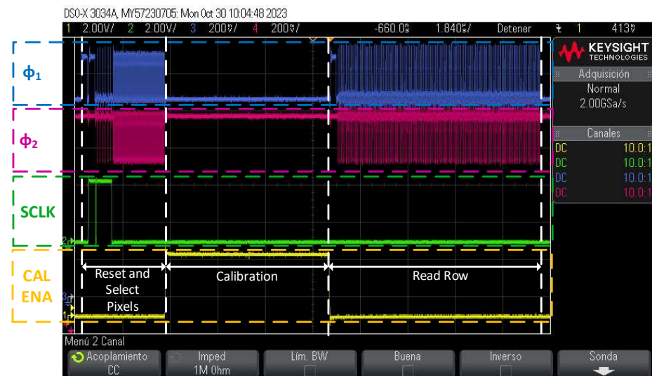
Figure 15. Reading and calibrating row sequence using oscilloscope capture.
