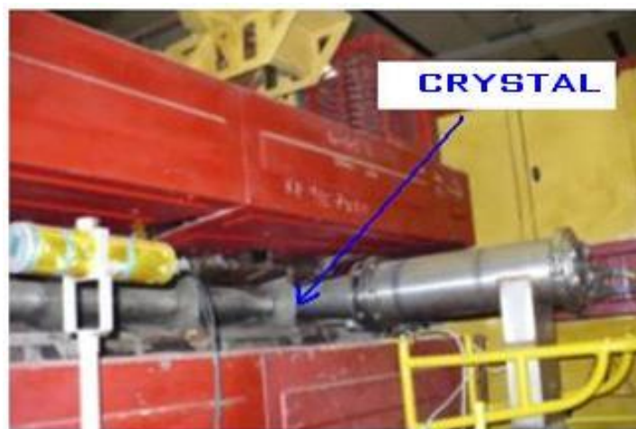
Figure 3. The extraction of a beam from U-70 ring by crystals 1 and 2 in a direction of beam lines N2 and N4.
