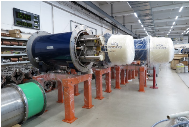
Figure 8: Assembly and preparation of magnets for shipment to the ring.
