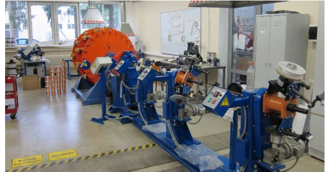
Figure 2: Cabling machine for the manufacture of a hollow composite SC cable.
