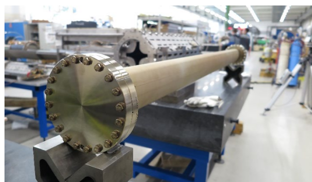
Figure 7: Checking the geometric parameters of the beam pipe and its further installation in a SC magnet.
