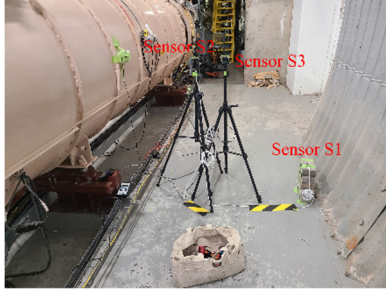
Figure 10: Experimental set up to measure the magnetic field during RHIC operation
