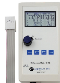
Figure 2: The MR3 sensor used to measure the magnetic field at the RCS location.
