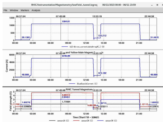
Figure 11: Stray magnetic field at close the DX magnet of sector 12 during RHIC operation, sensor 1M refers to the field magnitude at sensor S1.
