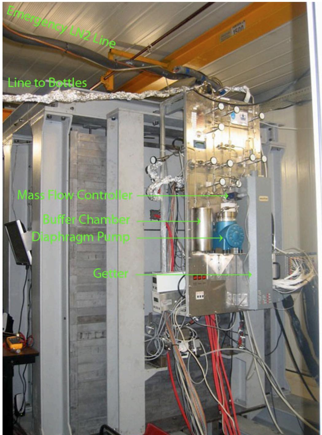
Figure 6.9: XENON10 gas system panel, which was largely developed by members at Coimbra University.
