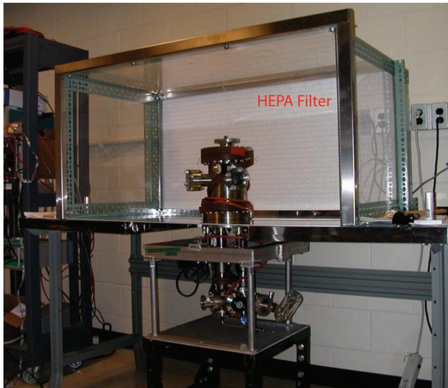
Figure 4.18: Clean bench with HEPA filter unit and blower.
