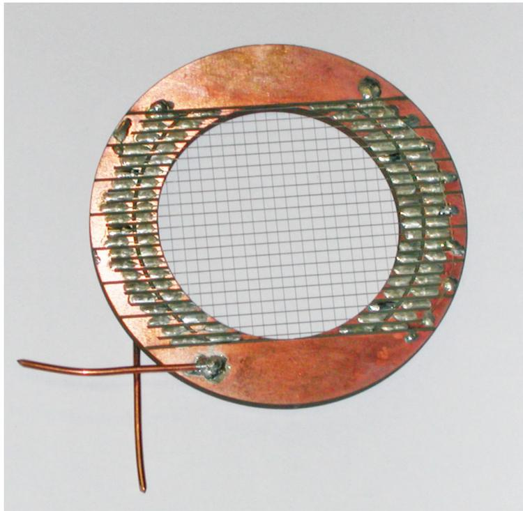
Figure 4.11: A Cirlex ring with laser etched individual pads. The wires are BeCu 125  $\mu\text{m}$ .
