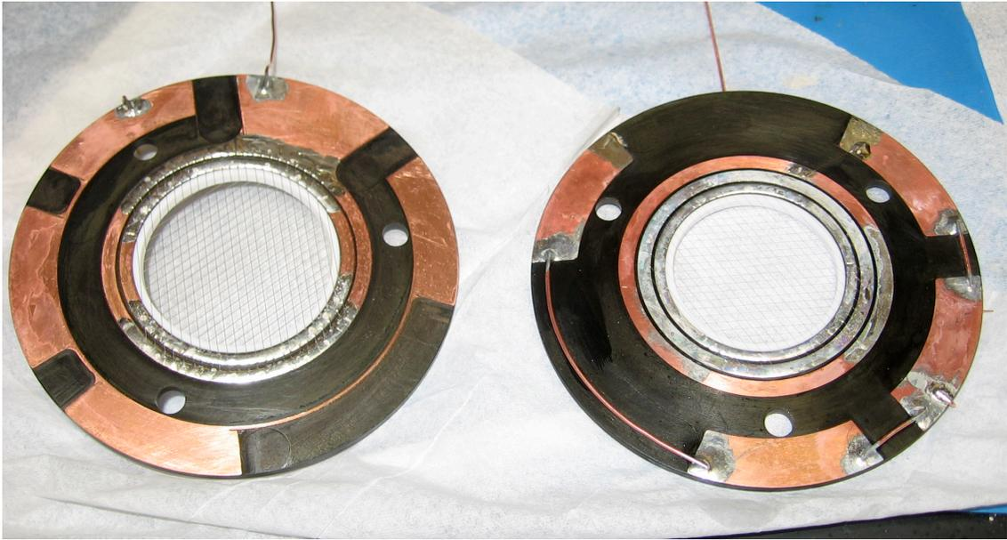
Figure 4.13: The Cirlex rings with 125  $\mu\text{m}$  (left) and 40  $\mu\text{m}$  (right) wires. The four on the periphery are the plates of the liquid level monitoring capacitor. Rings of this form were used for most of the measurements described in this thesis. In the center of each ring is a PTFE reflector.
