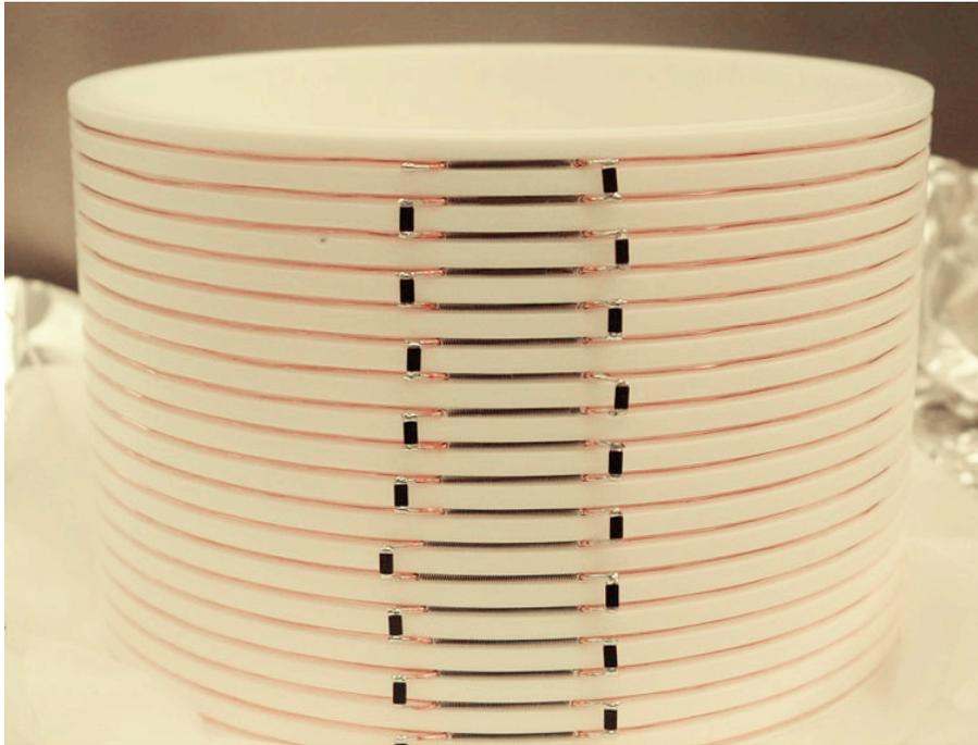
Figure 6.5: Copper field shaping rings with high voltage divider on the PTFE tube.
