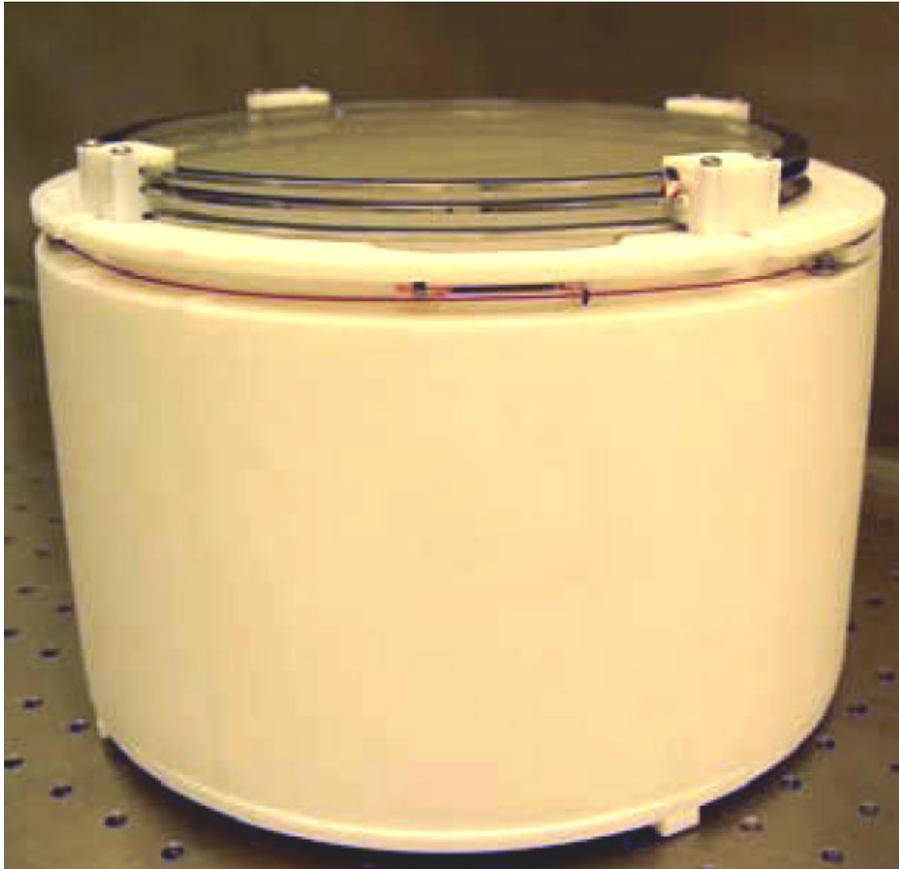
Figure 6.4: View of the top three of the electrode meshes and the outer PTFE ring.
