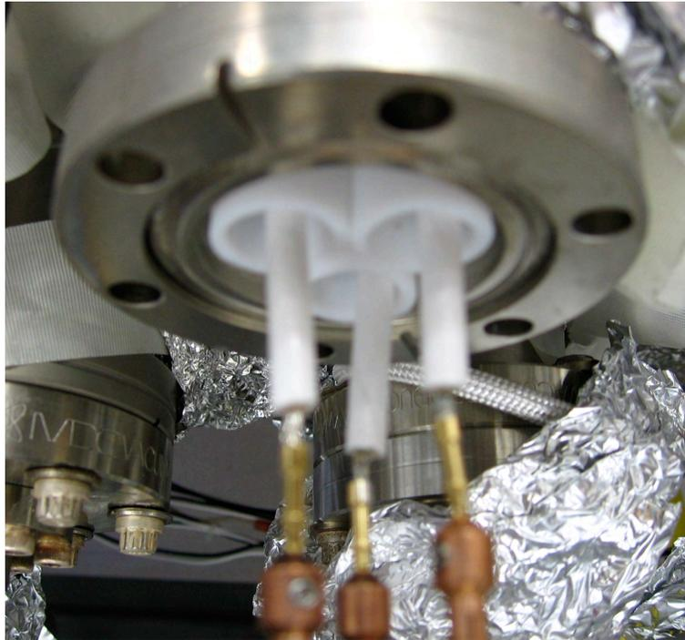
Figure 4.17: The PTFE tube insulating the connection between the Gortex wire and high voltage feedthrough.
