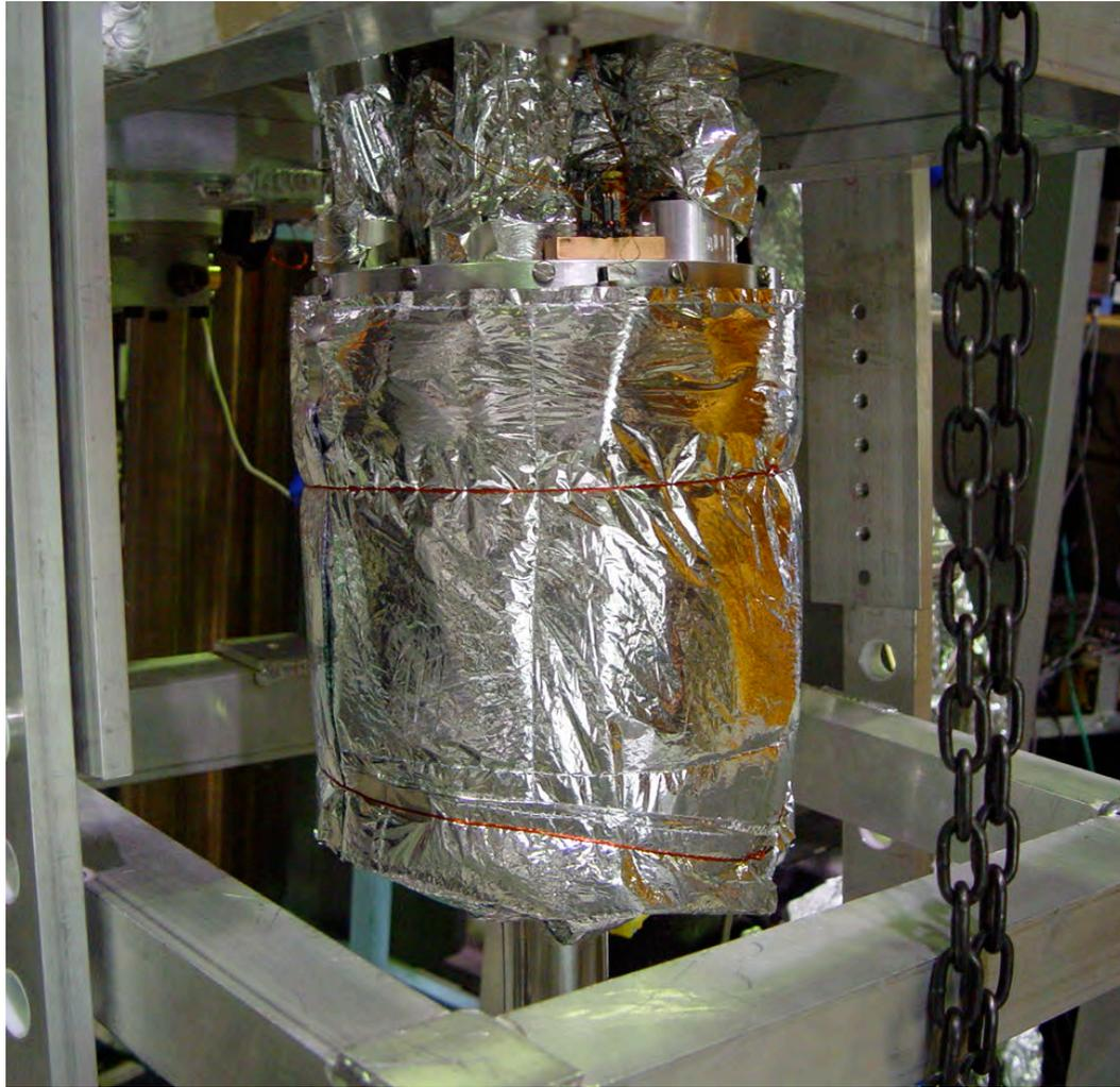
Figure 4.4: The radiation can covered with 10 layer aluminized mylar. The Vespel rods and stainless steel bellows have also been covered with the insulation.
