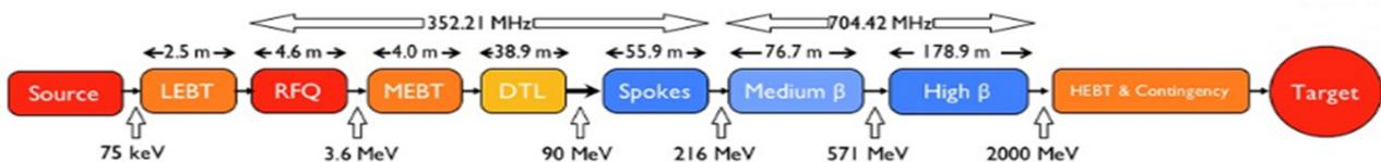
Figure 1: Schematic of the ESS Linac.
