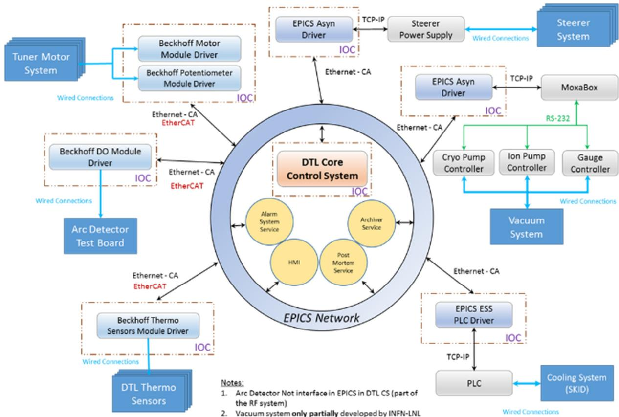
Figure 3: The scheme emphasizes the different technologies used for each functional sub-system to design the DTL control system.
