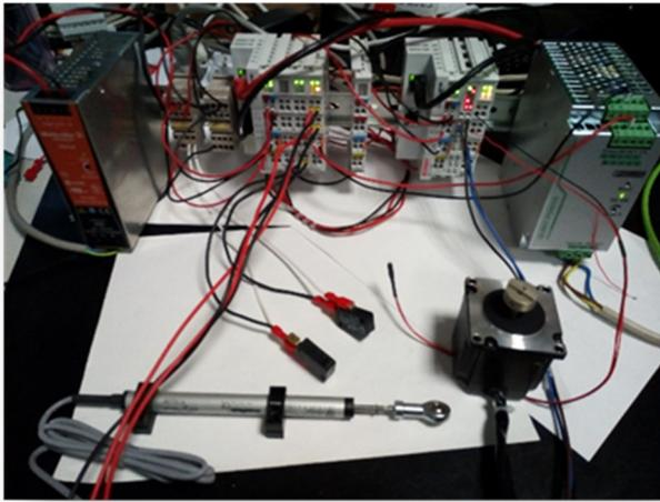
Figure 4: Test bench for the tuner system.
