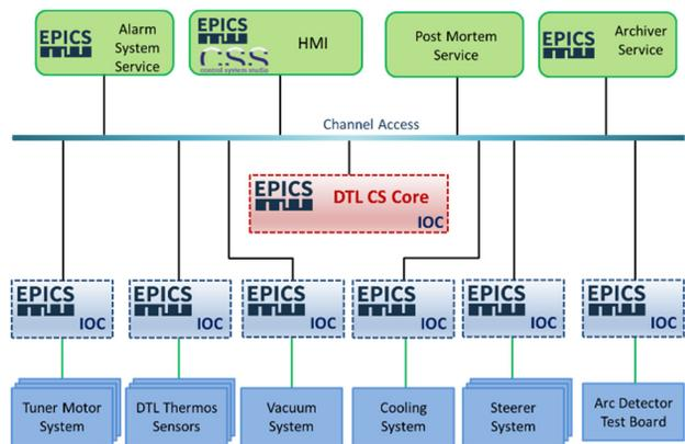
Figure 2: DTL Control System Architecture.
