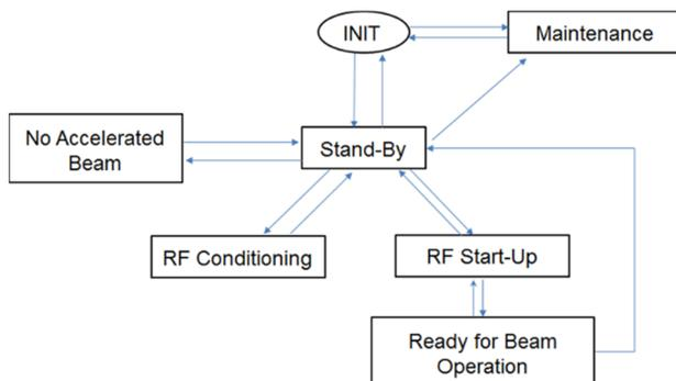
Figure 5: DTL-tank state machine schema.
