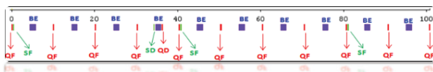
Figure 1: Schematic layout of magnets in one super period of booster lattice. The blue, red and green boxes represent dipoles, quarupoles and sextupoles respectively.
