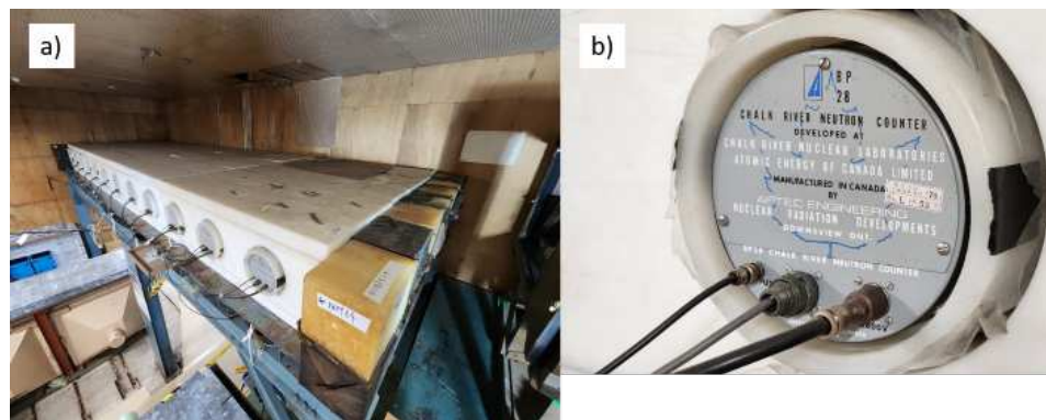
Figure 7. Photograph of the neutron monitor located at Mt. Norikura cosmic ray observatory (2778 m) (a) and the BF 3 counter (Chalk River neutron counter) (b).
