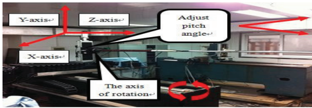
Figure 2: Hall-Probe Measurement Facility.
