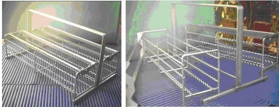
Fig. 5.30 – Last generation of film holders that can host 60 films at once in two independent modules.
