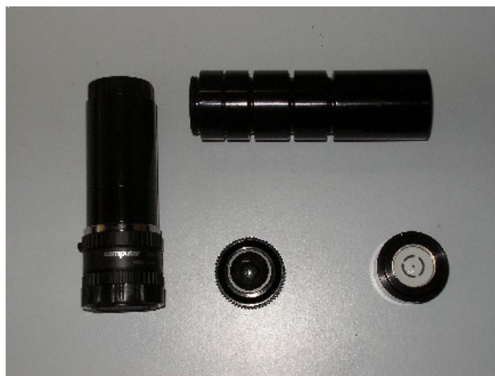
Fig.5.47 – Commercial spacers and lens holders, on the left there is also the light module for reference circled dots with the custom mask.
