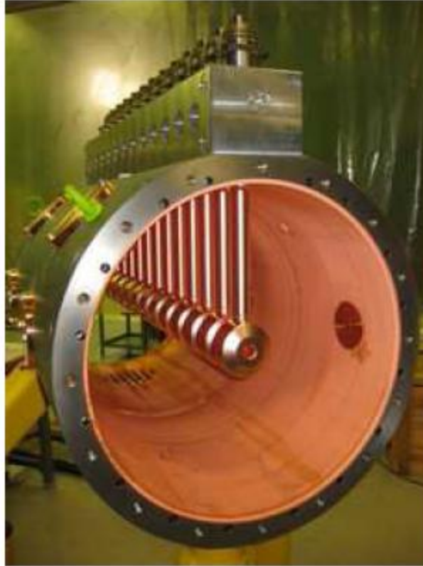
Figure 22 : DTL prototype in the assembly stage.
