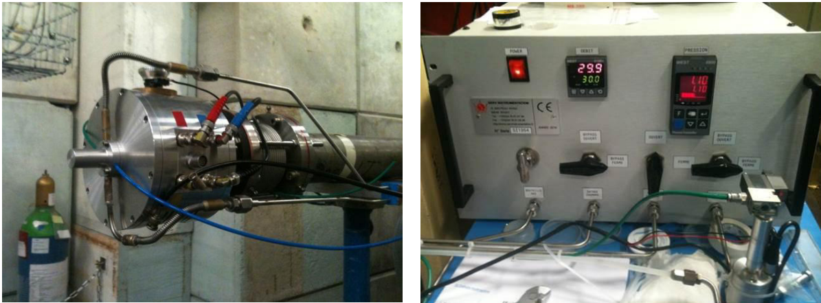
Fig. 2. (Color online) Left: The new LICORNE neutron source converter; Right: The hydrogen gas pressure and flow control system.
