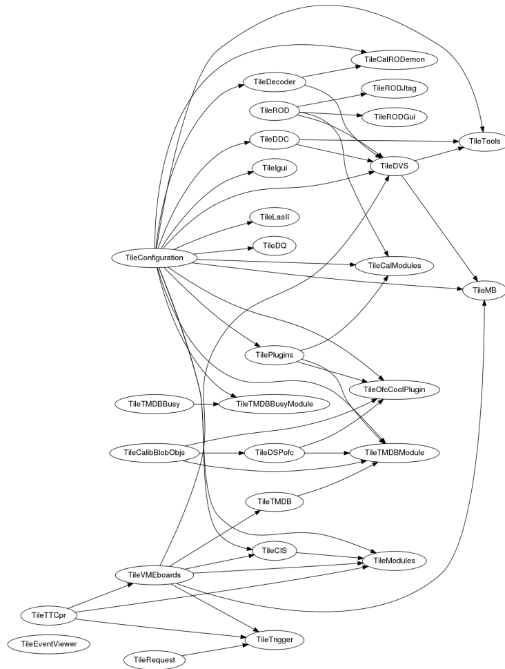
Figure 3.5: A graph showing all packages currently available in the TileCal Online software release. The total number of packages is 29 and most of them depend on the TileConfiguration package.
