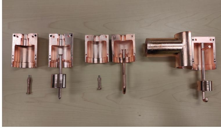
Figure 4.24: 3D-printed epoxy (Accura 48 HTR) and copper-coated HOM coupler prototypes. From the left to the right: probe-type, hook-type, and DQW-type PERLE couplers [123]. The figure falls under the Creative Commons Attribution 4.0 (CC BY 4.0) license ( https://creativecommons.org/licenses/by/4.0/ ).
