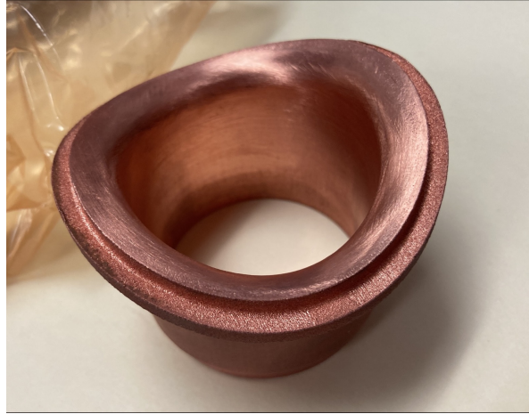
(b) 3D-printed Cu port after polishing
