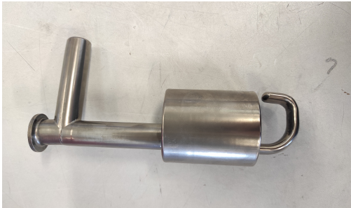
(a) Ti 3D-printed DQW coupler
