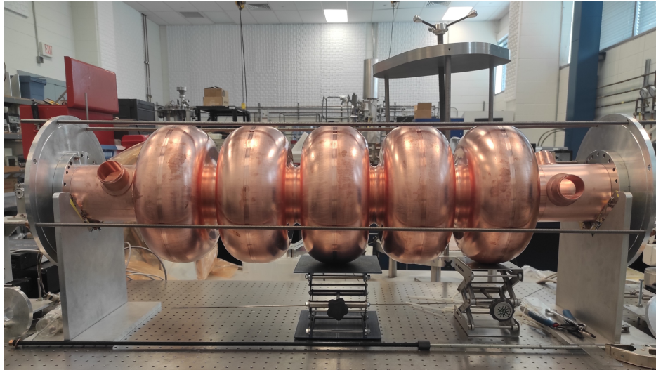
Figure 6.12: Cu prototype of 801.58 MHz PERLE cavity fabricated at JLab.
