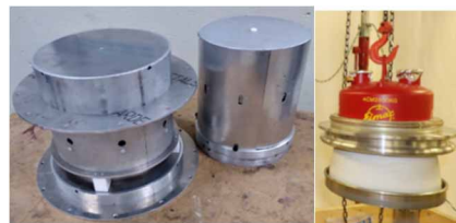
Figure 1: Surrogate tetrode made to the mechanical dimensions of the actual 4CM2500KG tetrode (left) and the added resistances to emulate the electron beam currents (right) photo of 2.5 MW high power 4CM2500KG tetrode.
