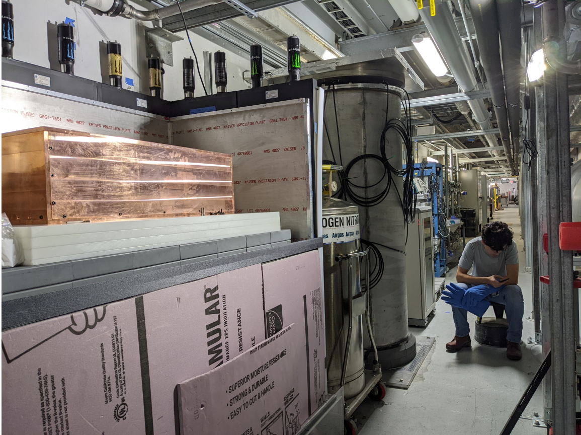
Figure 6.4: A photograph of the Ge-Mini detector system, sitting inside of Neutrino Alley, on the day of the first cool down, on November 28, 2022. The system was in a state of partial assembly. The copper box, which surrounds the detector cryostats, is fully assembled. Visible inside the partially assembled shielding are the four-inch layers of plastic and lead shielding, as well as the active muon veto system.
