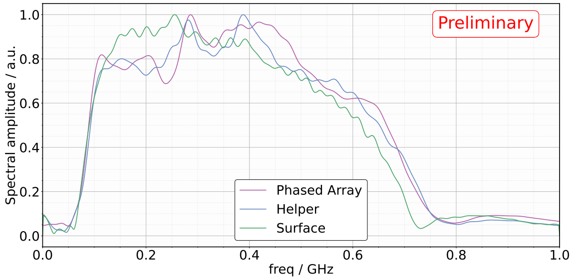
Figure 2: Normalized lab measurement of the system's frequency response. The response was measured at the RADIANT channel output corresponding to both deep and surface components. Note that since the phased array is the main trigger, this system response also includes a signal splitter.
