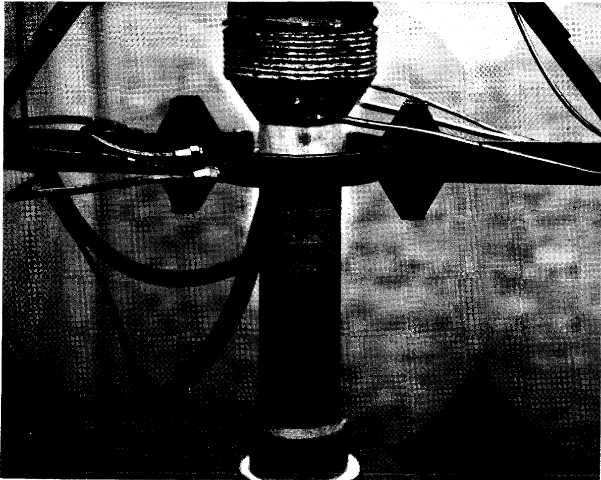
Fig. 13B Close-up of scale model brazing furnace, showing the ring burner moving down over the stacked parts of a short accelerator section.
