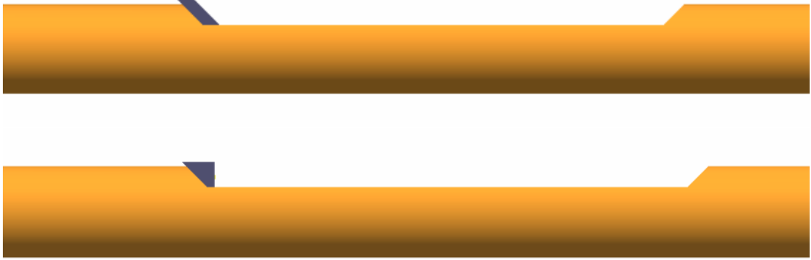
Figure A.7: Schematic of the Tungsten radiators (parallel above and trapezoid bottom) coupled with the 45^\circ window shape beam pipe.
