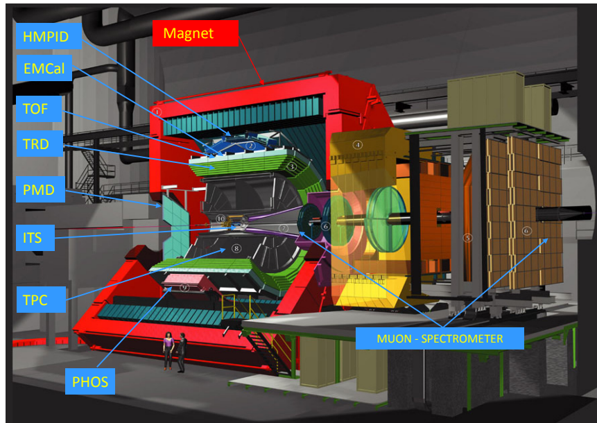
Figure 2.1.: The ALICE experiment with the detectors: HMPID (High Momentum Particle Identification detector), EMCal (ElectroMagnetic Calorimeter), TOF (Time-Of-Flight detector), TRD (Transition Radiation Detector), PMD (Photon Multiplicity Detector), ITS (Inner Tracking System), TPC (Time Projection Chamber), PHOS (PHOTon Spectrometer), Muon detectors
