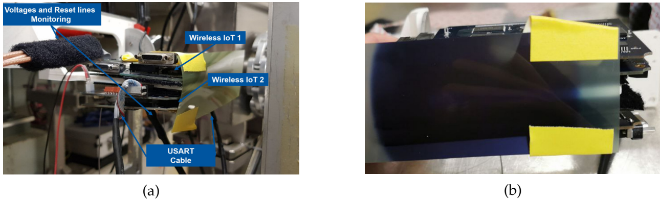
Figure 3.30: In Fig. 3.30a, the two Wireless IoT systems are mounted with their side part facing the source. They are stacked on top of each other to be tested together. In the figure, the different cables connected to increase the observability of the device are listed. A Gafchromic film was also mounted on the side of the two systems to check the effective irradiated area. At the end of irradiation, the targeted area was all black as visible in Fig. 3.30b, proving that the test setup was correct.
