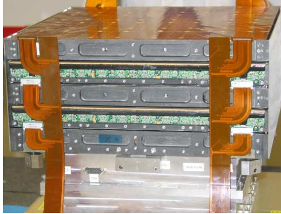
Figure 1: The GLAST Mini-Tracker, just before the assembly of the last sidewall. The front-end electronics boards (two are visible in the picture) are mounted on the sides of the trays - to minimize the gaps between adjacent towers - and connected to the silicon detectors by means of 90^\circ pitch adapters. The power, control, trigger and data pass through 8 flex cables (two per side), providing full redundancy against single point failures to the electronics system [2].
