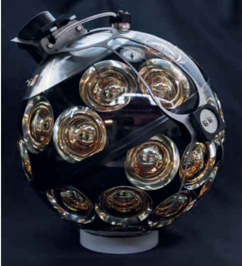
Figure E.4: The KM3NeT optical module containing sensitive light detectors.
