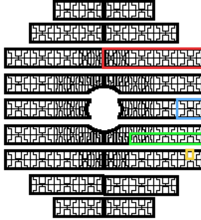
Figure 5.3: Visualization of chamber 6 showing its different substructures: DE (red), PCB (blue), BP (green) and MANU (yellow).
