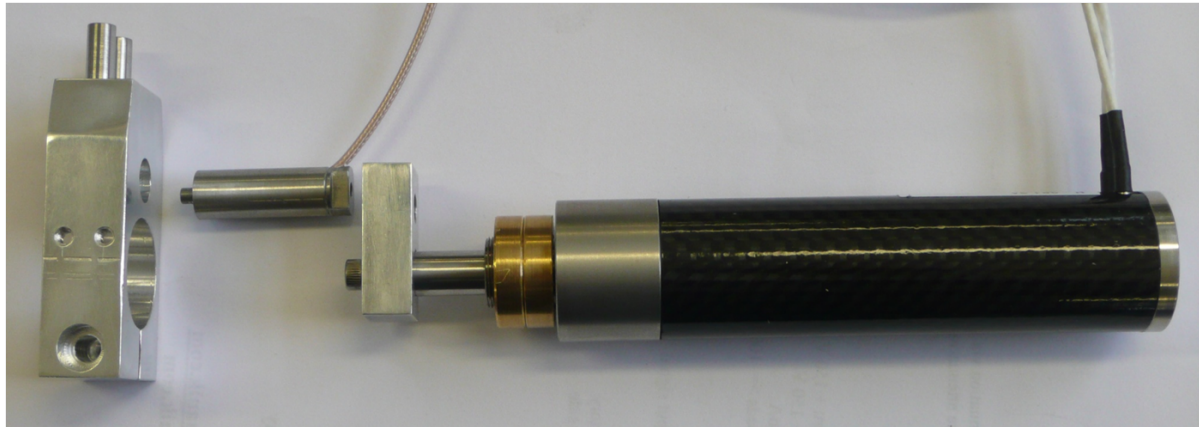
Figure 2. The new low-voltage stepper motor and piezoelectric actuator, along with supports, being used in the DPUNS device.
