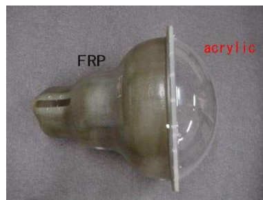
Figure 3.10: PMT case to prevent a chain reaction in the case of an imploded PMT.
