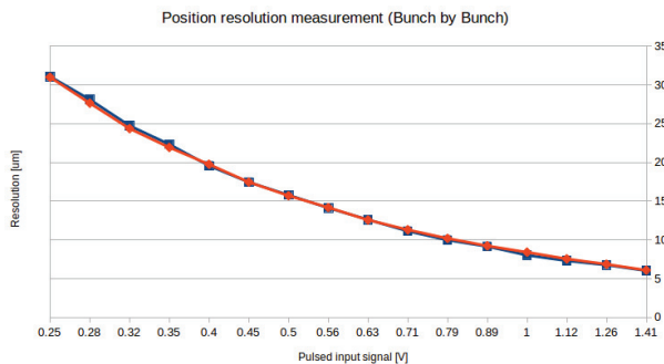
Figure 8: Position resolution (15 dB dynamic range / FWHM=30ns).
