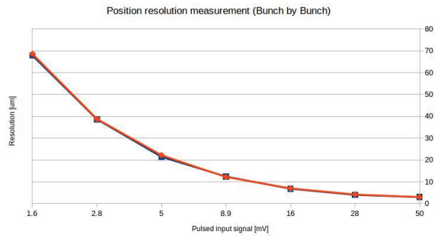
Figure 9: Position resolution (30 dB dynamic range / FWHM=100ns).
