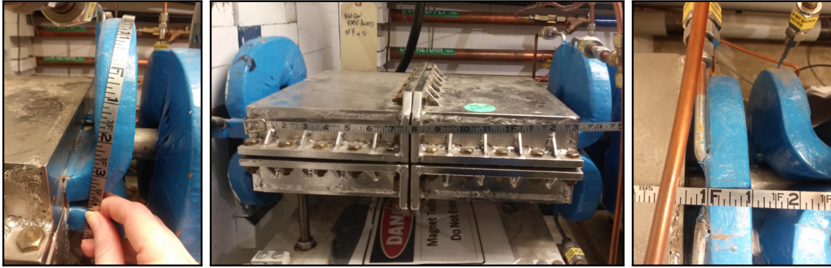
FIG. 50: Coarse physical measurements being taken of the raster magnets.
