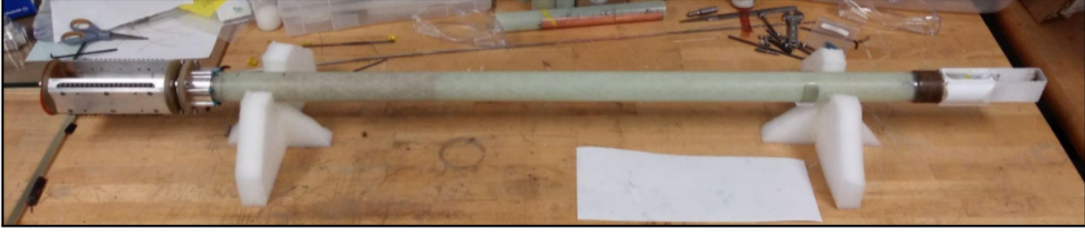
FIG. 29: The movable bath trolley which runs within the insert to transport target cells in and out of position within the detector. The left-hand side of the image is the upstream end of the trolley terminating with the trolley base (see Fig. 33), which attaches to the movement tethers and houses the ball-bearings by which the trolley glides. The right-hand side of the image is the downstream end of the trolley terminating with the Kel-F bath (see Fig. 34), which holds the target cells. Connecting the two ends is the trolley body made up of two concentric cylinders containing the liquid level probes and thermal sensors. Liquid helium fills the space between the cylinders as well as the Kel-F bath.
