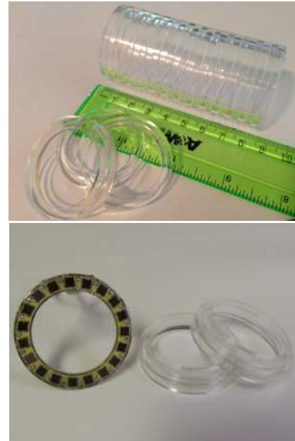
Figure 6. A prototype of the multifoil fission fragment tagging detector based on thin scintillator foils. Top panel) Acrylic light guide rings. Bottom panel) A ring of silicon photomultiplier sensors that will convert the light to electrical signals.
