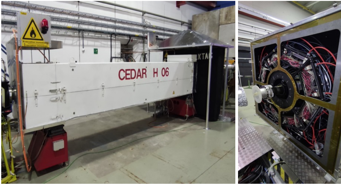
Figure 3.26: CEDAR-H installed in the NA62 beamline (left) and the KTAG photon-detection system reassembled at the upstream end of the vessel (right).
