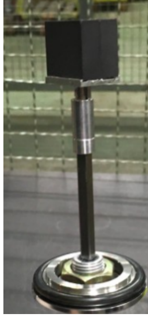
Figure 4.6: The thin carbon target used in the 90 GeV/ c proton-carbon dataset analyzed for this thesis.
