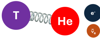
Figure 1.4: Initial beta-decay of \text{T}_2 resulting in a {}^3\text{HeT}^+ ion, electron, and electron antineutrino
