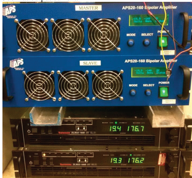
Figure 5: Bench testing with negative output current.
