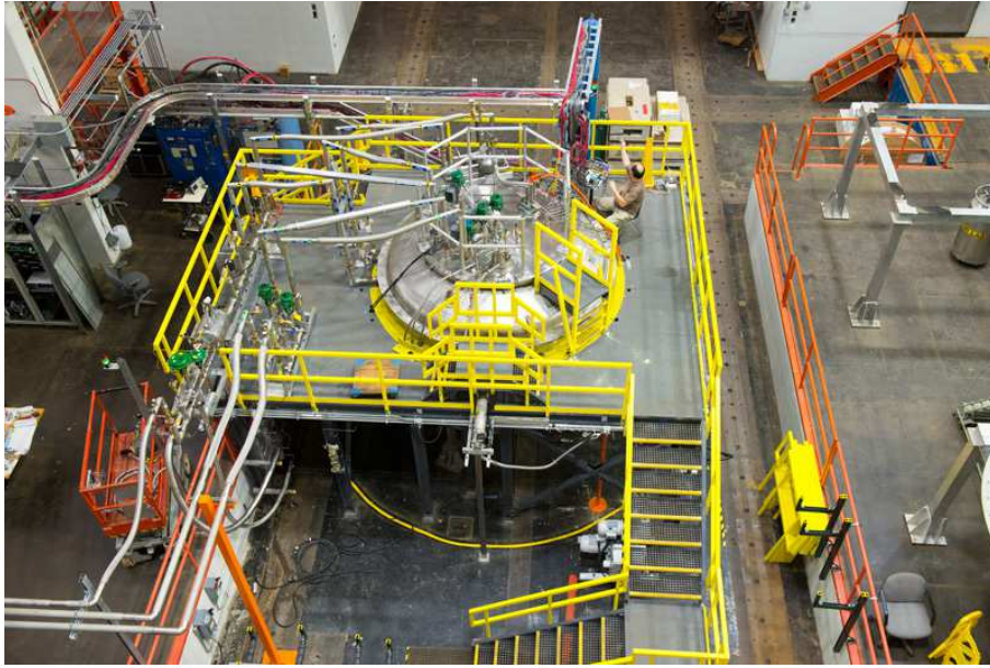
Figure 2. Photograph of the existing experimental installation, including the associated work platform and cryogenic infrastructure. The vacuum vessel was previously used as a liquid helium test stand for solenoids for the Mu2e project. While the final design of Colossus replaces this vacuum vessel with a new vessel of similar design, the work platform will be reused. Picture credit: Fermilab
